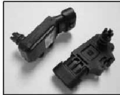
Absolute pressure/intake temperature sensor for intake manifold
